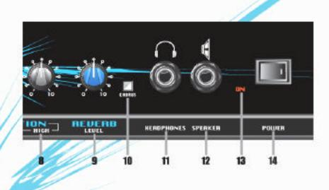
**9: REVERB LEVEL:** Use this control to adjust the amount of reverberation: in its full counter clockwise position the signal will be "dry" (without any reverb). As you rotate the control clockwise the amount of reverberation increases.
